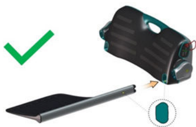
Correct assembly (first mount the backrest)
