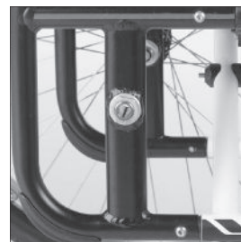
MA 114 Drive wheel adapter, permanently welded
