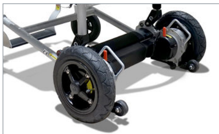
Anti-tippers keep you safe on hills and inclines.
