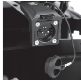
EU043 External magnetic charging receptacle
