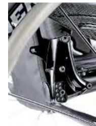
// NTR030015 Backrest, angle-adjustable, fold-down
