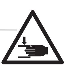
Caution must be exercised when moving or collapsing the anti-tippers, particularly during manual adjustment or activation. As a result of the high spring force required there is a risk of crushing between the holding rod [21] and the clamping piece [22].
