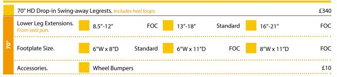
The 8"W footplates may cause interference with seat widths less than 19".
